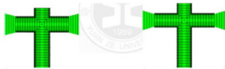
Figure 17 Primary runner and sub-runner before and after modification
